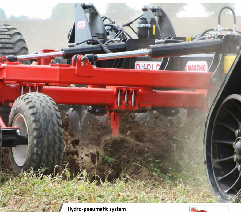
The auto-reset circuit with double nitrogen accumulator and safety valve prevents frame damage and reduces downtime resulting from having to replace the shear bolt. Once the obstacle is overcome, the system brings the shank back to its working position. The nitrogen accumulator capacities are 7.5 I for the hydropneumatic models with 5 shanks and 17 I for the versions with 7 and 9 shanks.
