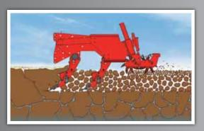
The subsoiler models PINOCCHIO, ATTILA, ARTIGLIO and ARTIGLIO MAGNUM are equipped with a double counterrotating spike roller having Ø of 140 or 220 mm and a variable number of blades from 16 (for 1.30 m versions) to 96 (for 5 m versions). The high number of spikes and the large diameter improve residue sizing and incorporation, clod shattering and soil levelling.
